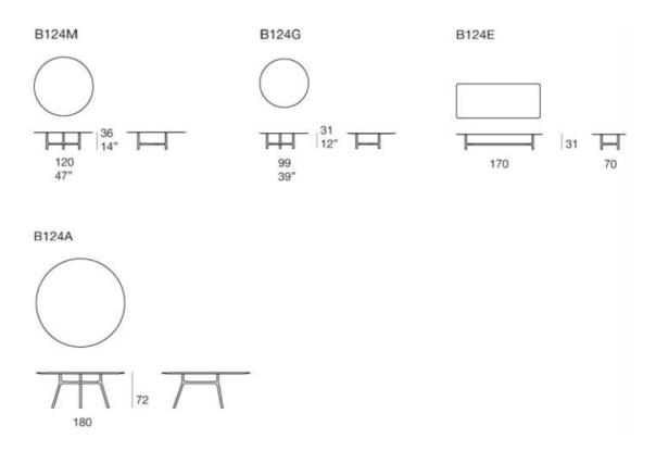
**Base**: molded aluminium joints and profiles in extruded aluminium matt laquered in avorio or grafite colour; plastic spacers.
