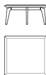
56701 Tavolino quadrato base in frassino, top marmo Square low table base in ash wood, marble top cm 80 x 80 x h 37 in 31 1/2 x 31 1/2 x h 14 1/2
