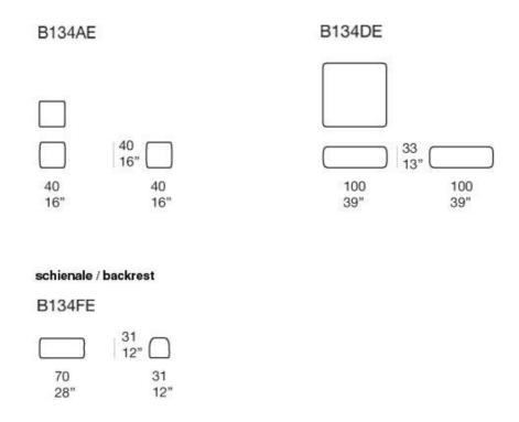
**Structure**: polystyrene spheres encased in a polyester covering. Insert in expanded polyurethane in a water repellent polyester covering.
