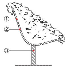
**Structure** Injected flame-retardant foam ① over internal steel frame ②. Rotary base in grey varnished steel metallized grey ③ and glides in neoprene rubber.
