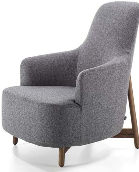
*Armchair with frame in solid canaletta walnut and cover in the fabrics of the collection. The cover is removable in fabric and fixed in leather. It is possible to combine different fabrics for the outer and inner parts of the upholstered structure. Inner shell in poplar plywood and solid fir wood with belted seat. The padding is in crush-proof polyurethane with different densities.*
