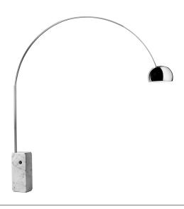
Floor lamp providing direct light. White Carrara marble base. Satin-finish stainless steel telescopic stem. Pressed, polished and zapon-varnished aluminum swiveling and height-adjustable reflector.
