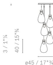
Each cable is adjustable in length up to a maximum extension of 250 cm.
